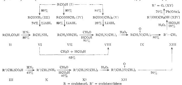
The individual steps required for the degradation of I to cyclohexene in about 52% over-all yield, via the successive application of the Schmidt reaction,<sup>11</sup> the Eschweiler-Clarke reaction<sup>12</sup> and the Cope amine oxide pyrolysis,9 have already been described. In the chart several alternative degradations of I as well as degradations of II and III are outlined.
